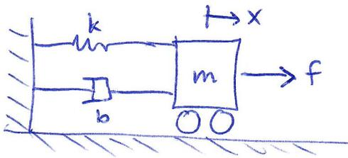
We have:  $m = 1 \text{ kg}$ ,  $b = 1 \text{ N}\cdot\text{s/m}$ ,  $k = 10 \text{ N/m}$ .
